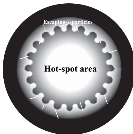
Figure 6.1. Schematic picture of the reduced self-heating of the hot-spot area from prematurely escaping \alpha -particles.
